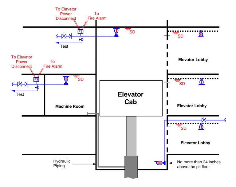
Figure 6-10 Holeless Hydraulic Elevator
