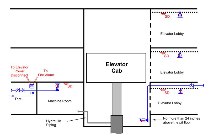
Figure 6-9 Direct Plunger Hydraulic Elevator – Hydraulic Supply Piping Extending above the Second Finished Floor Elevation
