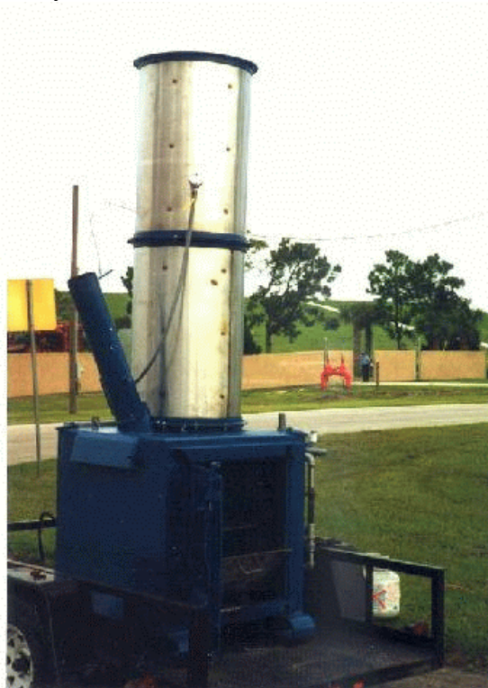
Double Chamber burn unit designed by REMTC
