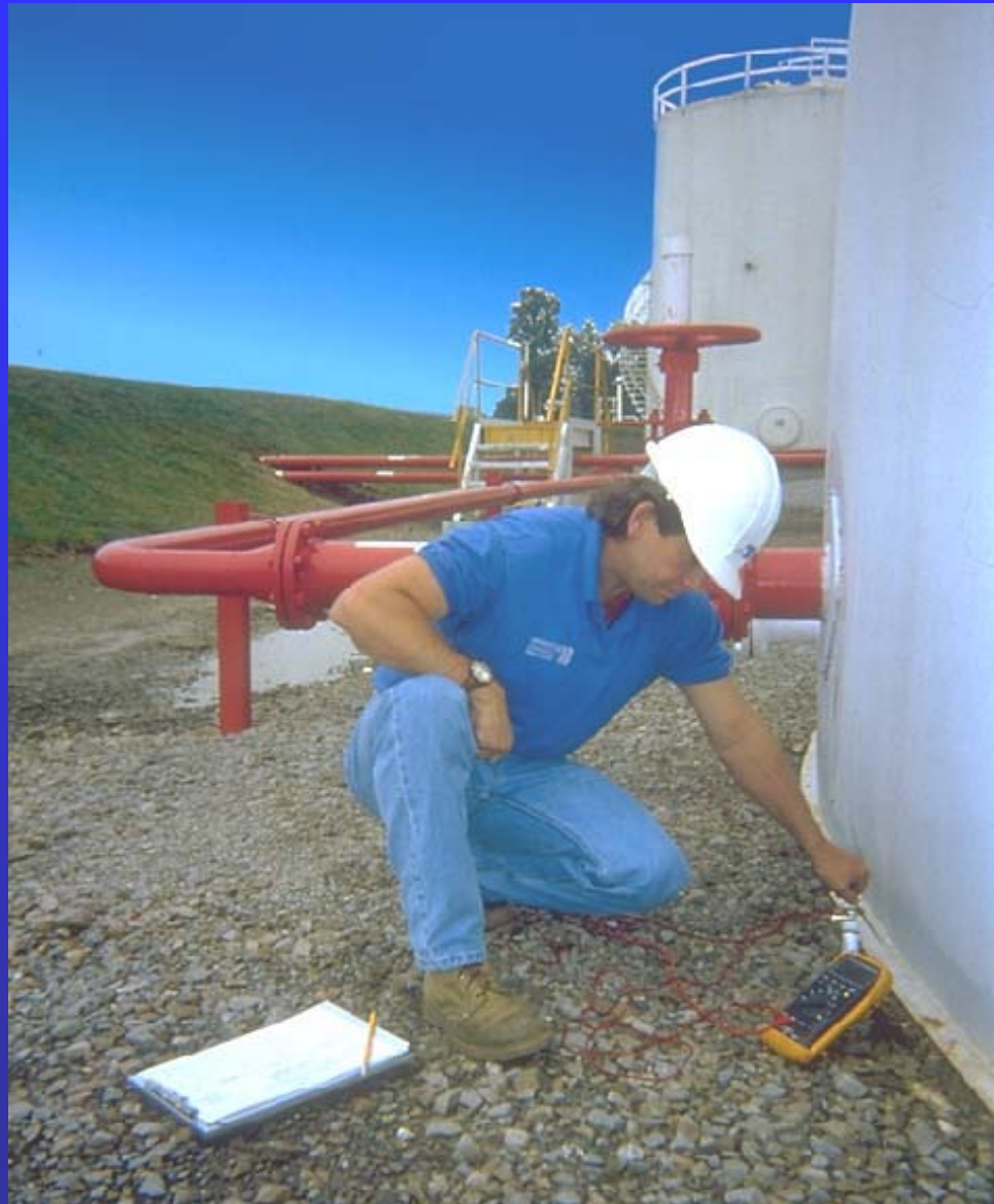
Annual Cathodic Protection Survey
