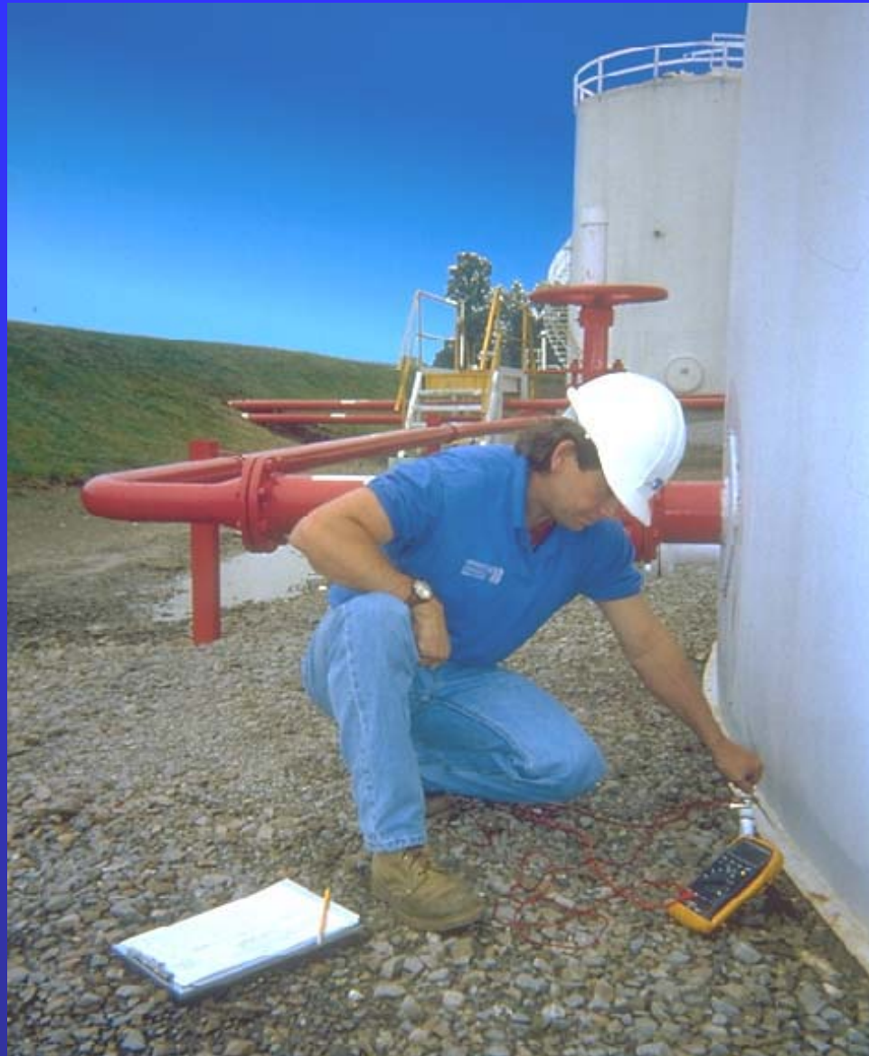
Annual Cathodic Protection Survey
